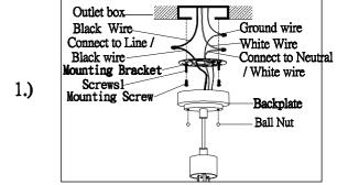
Step.1: Remove mounting bracket from fixture and install to electrical box. Wire fixture to wires in outlet box. Copper wire is for Ground.
