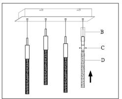
4. Carefully remove packaging from fixture.5. Adjust wire length to desired mounting height, and tighten strain relief screws to secure.
