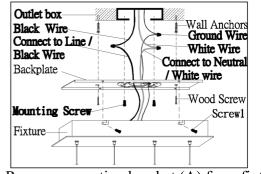
Remove mounting bracket (A) from fixture
