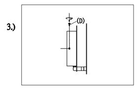
Step.3: Install fixture to bracket and tighten finials (D) at the ends of the canopy to secure.
